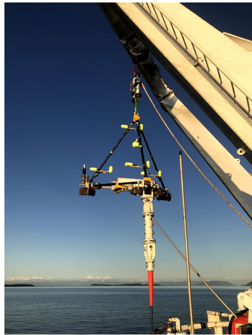
Figure 2.1: Deployment of an Underwater Listening Station (ULS) frame in Boundary Pass. Copyright of JASCO Applied Sciences.
